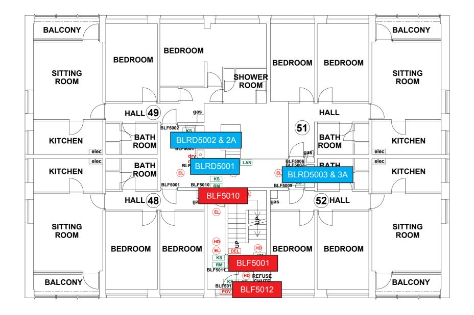
POV Permanently Open Vent Fire alarm sounder ('X' indicates integral flashing - Xenon light) CCTV CCTV Security Camera
